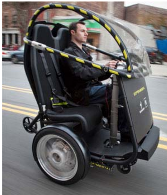
Figure 42. A version with two seats and one axle, based on Segway technology. Photo source: www.scientificamerican.com
