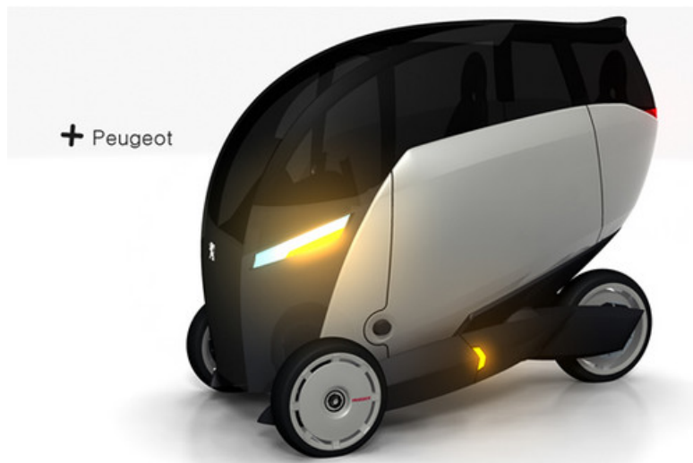
Figure 44. A design study called Peugeot plus, by David Vargas, for the Peugeot Design Competition 2007. There is room for two passengers. The length of the vehicle is 2.2 metres and the width is 1.2 metres. Photo source: http://psipunk.com/peugeot-brings-three-wheeled-eco-vehicles-to-style/
