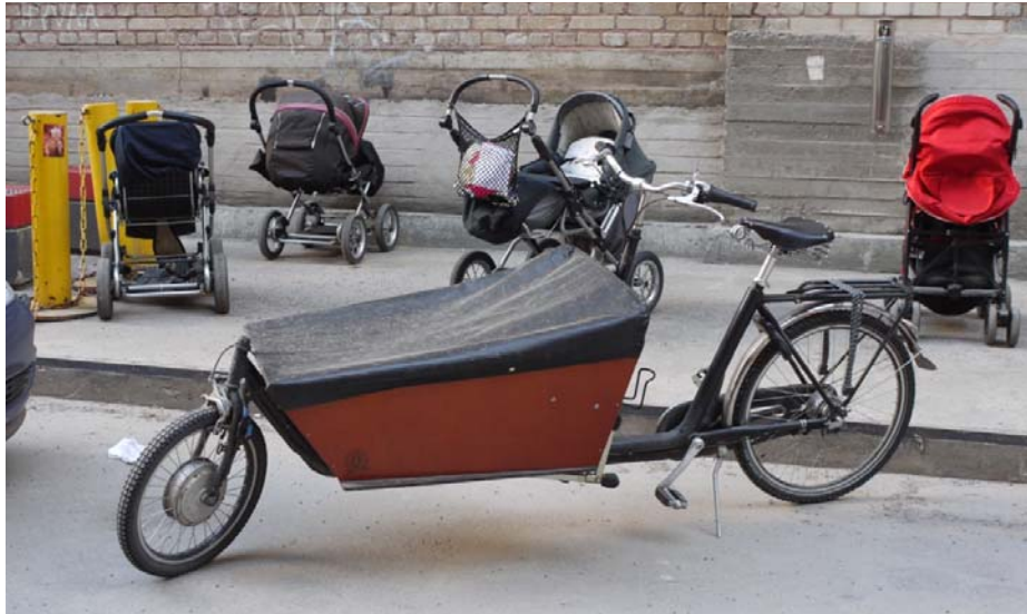
Figure 45. A bicycle equipped with a gargo box typical in Amsterdam. The version in the picture is a pedelec having the electric motor in the front wheel. Photo A. Alku 26.3.2011.
