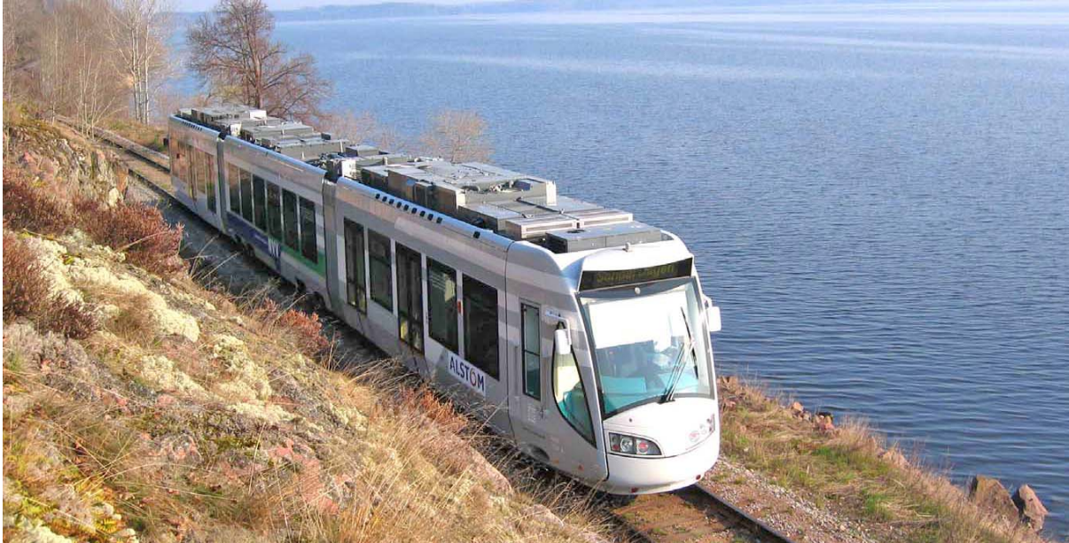
Figure 9. A hybrid tram on an unelectrified railroad track in Sweden in 2007. The Regio Citadis tram is built by Alstom for the city traffic in Kassel. Photo by Alstom.
