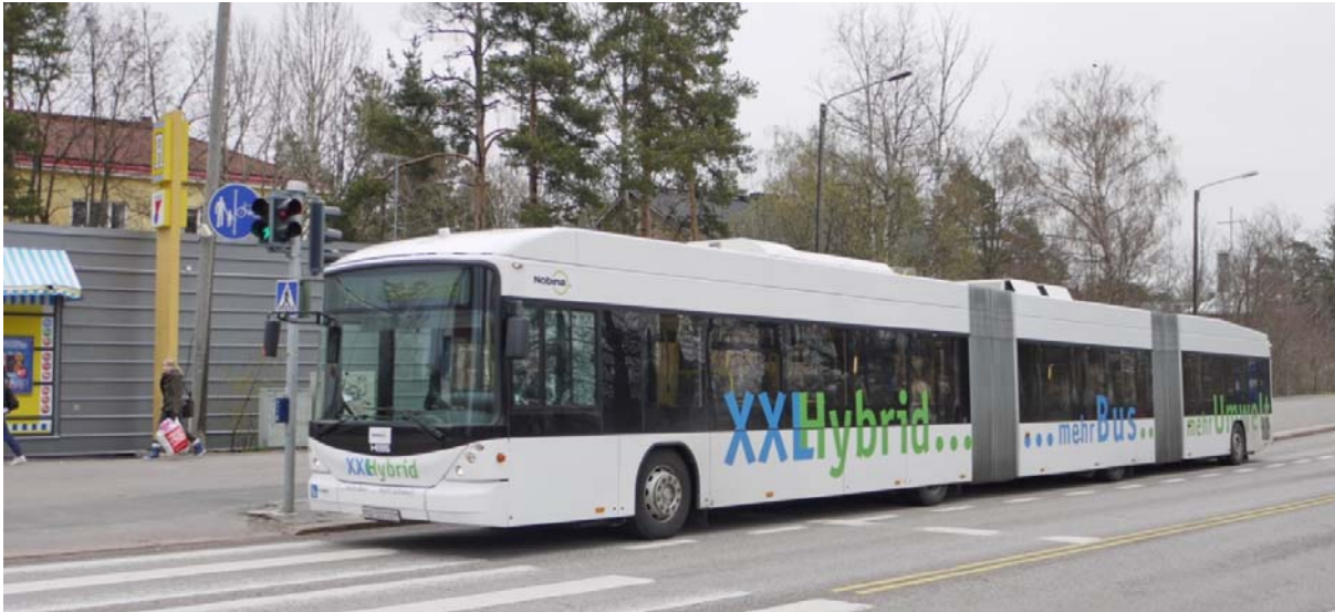
Figure 11. Articulated series hybrid bus with 2 pivoting joints, manufactured by Hess, in road test at Pitäjänmäki in May 2010. The bus is a modification of trolleybus; it has no trolley poles but there is an aggregate in the rear and supercapacitors on the roof. Diesel engine is constantly running during operation.
