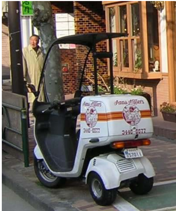
Figure 39. The Canopy model of Honda's Gyro moped was taken into production in 1990. The device includes a windshield, roof and a 62-litre cargo compartment. The engine, transmission and rear axle form a unit, which as a whole is fastened with a hinge to the chassis, which can tilt to the side while turning. Photo source: Wikipedia Commons.
