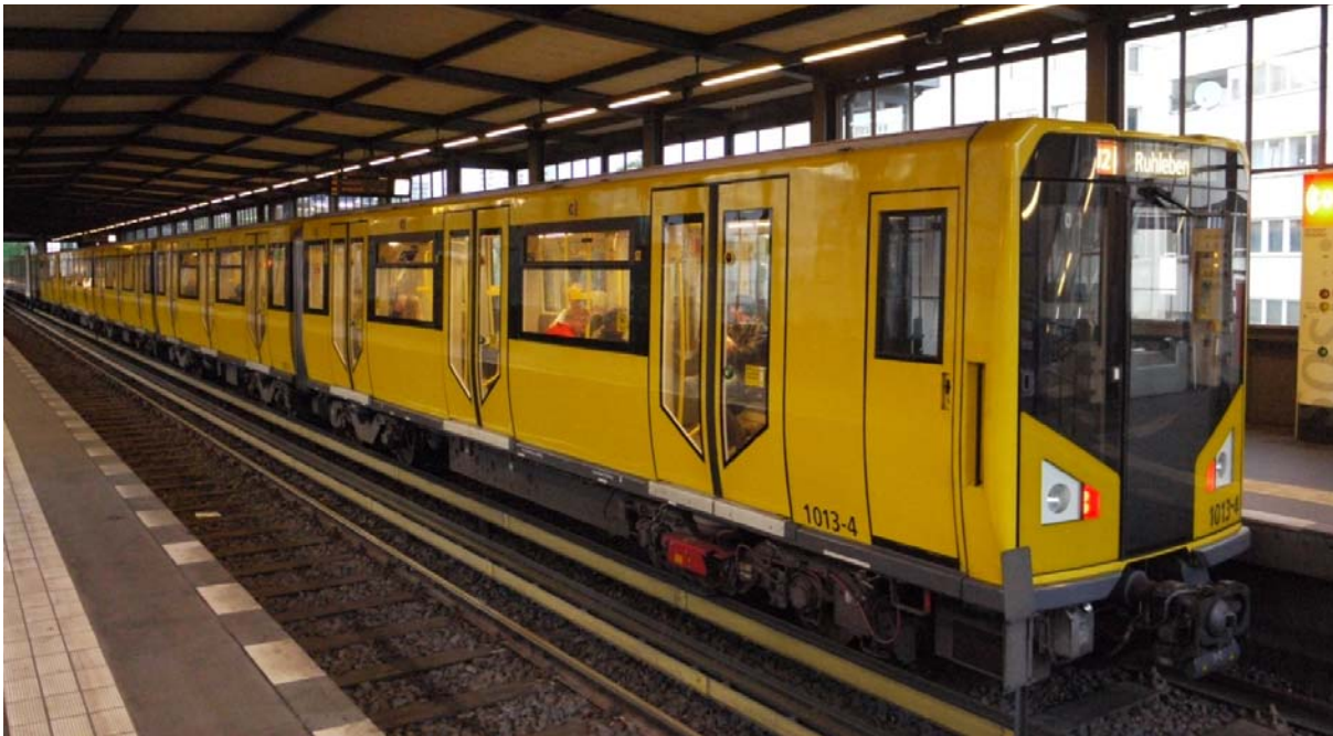
Figure 7. A metro train of the Berlin metro (U-Bahn), series HK, on the U2 line in September 2010. One train unit consists of four carriages, with a continuous passenger section from one carriage to another. The length of one unit is 51.6 meters and the trains consist of two units.
