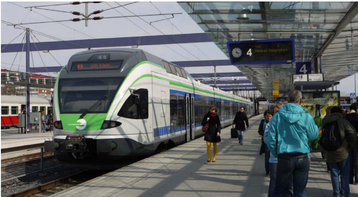
Figure 5. Motor coach "Flirt", i.e. series Sm5, operated by Pääkaupunkiseudun junakalusto Oy at the Leppävaara train station in April 2010. The train consists of four carriages, with a total length of 75.2 meters.
