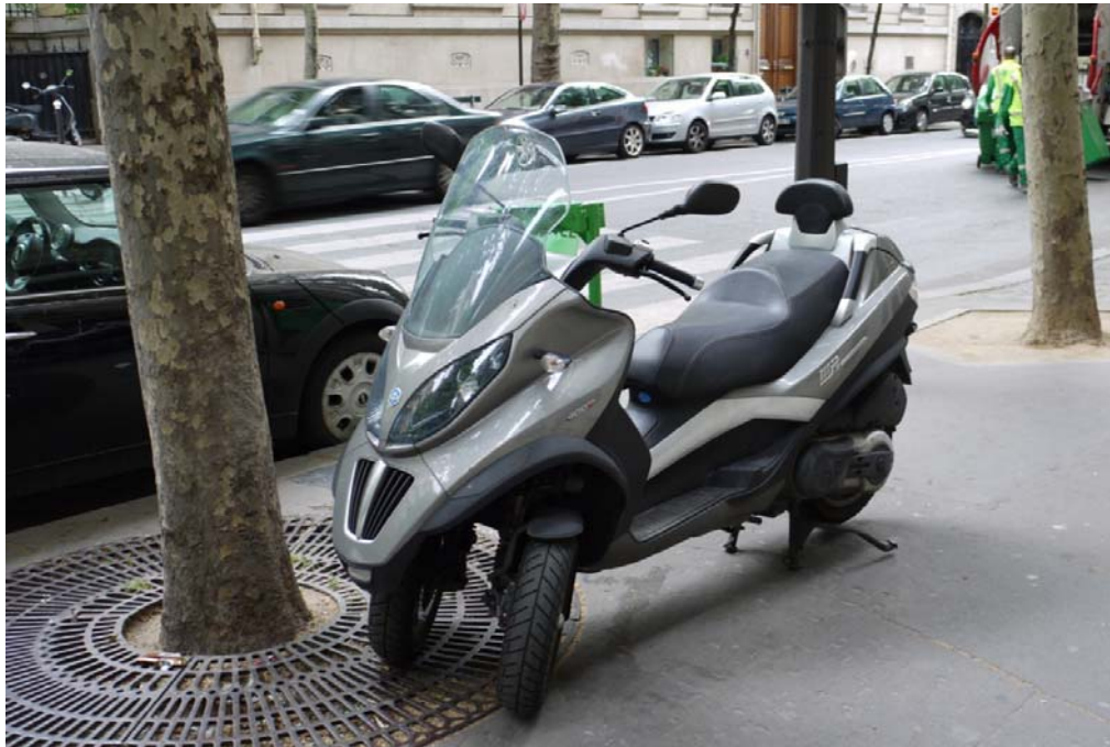
Figure 38. The 3-wheeled Piaggio scooter. The model has been parked with the help of a kickstand, even though the front suspension can be locked into standing position for parking.
