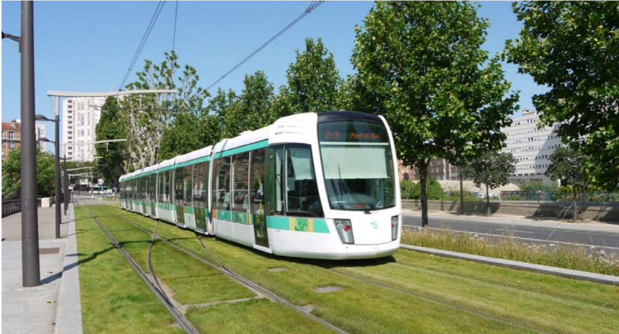
Figure 6. Alstom Citadis 402 tram of Paris tram line T3 in June 2010. The tram has seven parts and its total length is 43.7 metres.
