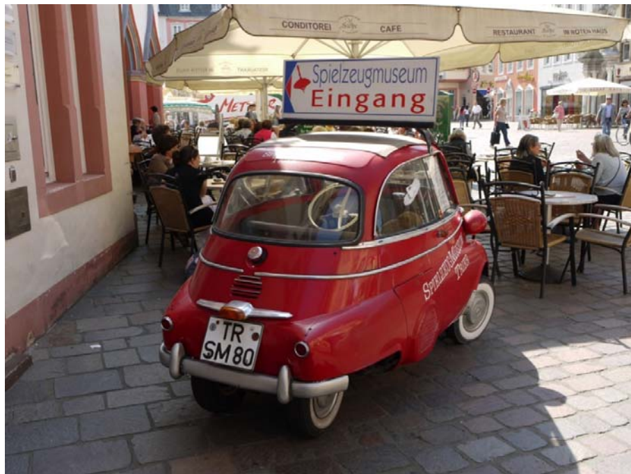
Figure 37. Microcars were common in the 1950s and 1960s when they were produced especially in France and Germany. Several models were 3-wheeled. However, the Isetta 250 model in the photo has 4 wheels, even though the gauge of rear axle is narrower than that of front axle. Photo 16.6.2010 A. Alku.
