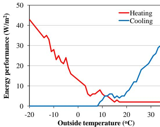
Figure 4.11: Specific energy performance of earth-to-air heat exchangers as a function of ambient temperature [45].
